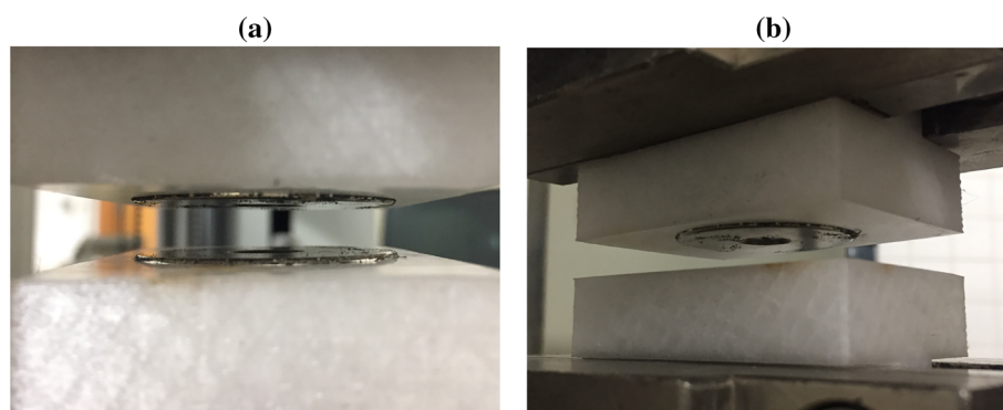
FIGURE 1 Experimental setup for the magnetic force–distance characterization. (a) Front view of the configuration with the magnets. (b) 3D view
